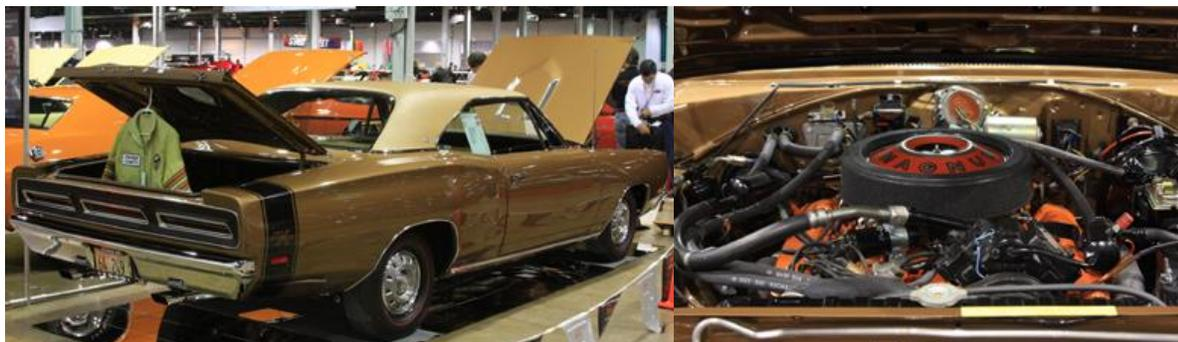
This is a 69 Coronet R/T owned by Chuck & Cindi Patula and has all numbers matching with original sheet metal and rare factory air, PS, PB, and wood grain wheel. Specifics; 440 4bbl engine, 727 auto trans, 8 3/4 3:23 gear ratio rear end and T-7 Dark Bronze Metallic color. This car features: Inline tube brake and fuel lines, parking brake cables, clips, & other detail underbody items.
