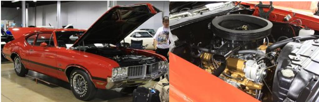
This is a very rare 1970 Olds Cutlass W31 Coupe, one of 116 made and one of only 12 with a bench seat. Specifics; original matador red paint, 350 CU in 325 HP engine, Muncie M20 4sp trans, and 3:23 Positraction. This rare beauty is 100% nut and bolt restored using NOS parts, original plating and finishes. This car features: Inline tube brake and fuel lines, parking brake cables, clips, and other detail underbody items.
